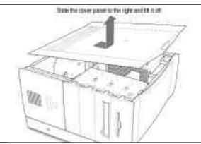
Sliding the cover panel to the right and lifting it off
